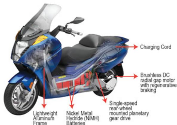
*Figure 2 – Vectrix Personal Electric Vehicle*
