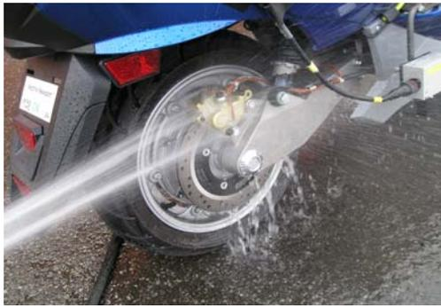
*Figure 9 – Vectrix brakes being soaked in water*
